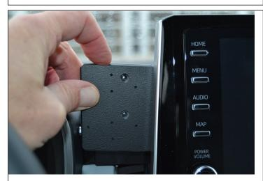
3. Align the holes in part 2 with the holes in part 1.
