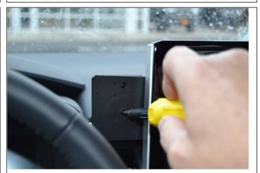
4. Screw the two parts together. Screw the screws tight but be careful not to over tighten the screws.
