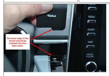
1. Clean the area where the ProClip will attach. Remove the tape covering from any tape on the mount. The lower edge of Part 1 of the mount should be inserted into the seam between the horizontal and vertical glossy hard plastic trim panels in the dash to the left of the information screen. See photo illustration.
