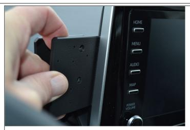
2. Once part 1 of the mount is in place, insert the thin right edge of part 2 of the mount (the face plate part) into the seam between the silver trim on the left side of the display screen and the back panel of the display. See photo.
